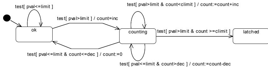
**Fig. 10.** Statechart diagram of refinement with counting and merged events
